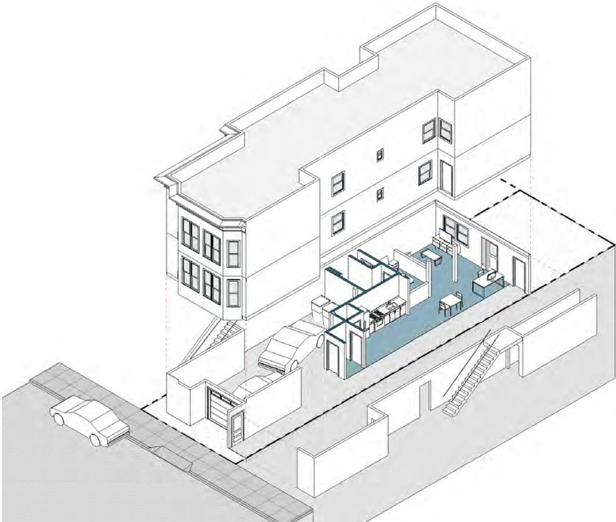
Ideally, the path is at least 36" wide and without obstructions that would interfere with the Fire Department moving equipment and personnel through the space in an emergency.
